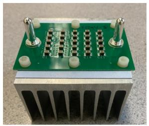
Figure 16 – 5x5 Array with small heat sink (HS1)
