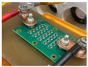
Figure 15 – 5x5 Array with no heat sink (NS)
