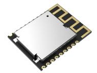
UART module MS48SF2 is based on m1805 Chipset. It is a small size (16×12×2mm) and stand-alone module with 12 GPIO. The data transmission between module and mobile phone can be achieved via operation of UART. With up to 60-meter working distance in open space, 512KB flash memory, etc., the data can be transmitted via Bluetooth
