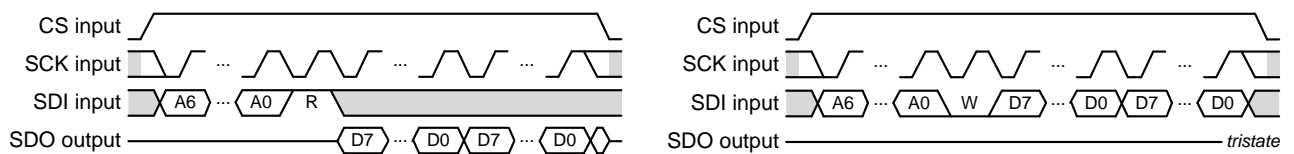
Figure 11: (burst) read/write SPI
