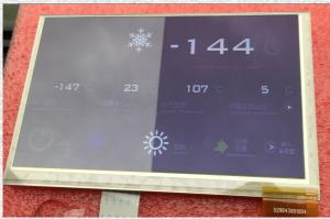
When boosting up brightness, not only number of LED chips but also other options to maximize the optical efficiency, such as DBEF, are considered to avoid excess power consumption. URT use high brightness backlight collocating with 3M DBEF film to increase LCM brightness, to avoid adding too much power and reduce heat.
