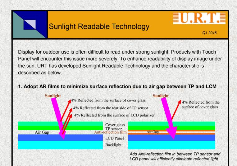
The AR film provides similar optical function as a full optical bonding, made by glue, while with a more competitive price point.
