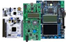
A full set of evaluation boards enables flexible prototyping as well as full STM32L4 evaluation. Commercial part numbers: NUCLEO-L476RG; STM32L476G-DISCO; STM32L476G-EVAL
